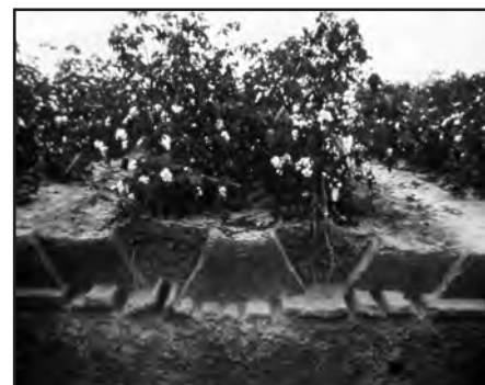
In this field the compacted layers of soil have been exposed by a backhoe, and the soil carefully picked away to reveal every tire imprint.
