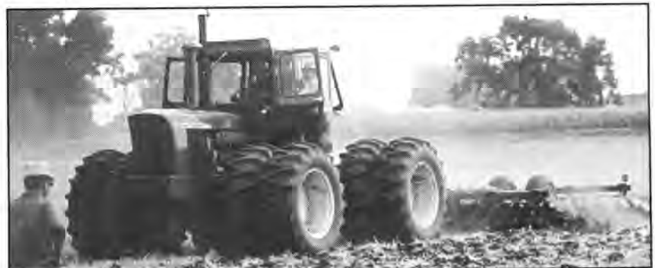
Large machinery can get the job done quickly, but the payback in terms of soil compaction is highly deleterious to subsequent production.
