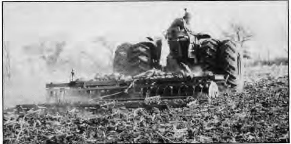
The disk harrow incorporates residues in a shallow layer, and according to Faulkner is an appropriate tool to emulate natural laws in many situations. It is a step up from the plow.
