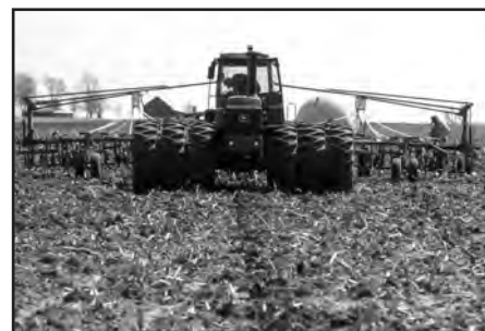
Heavy machinery traffic greatly compacts soil, especially when it is wet.
