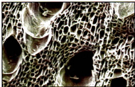
Biochar is highly porous, as seen in this close-up picture.
