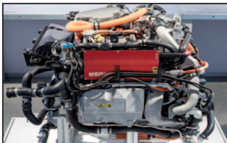
This BMW diesel engine runs just like a conventional reciprocating diesel engine, except it is powered by hydrogen.
